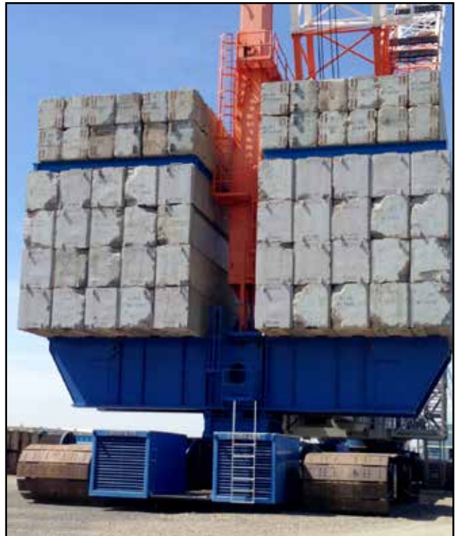
Counter weight for the Transi-lift, which is manufactured in Pasco by Operating Engineers
