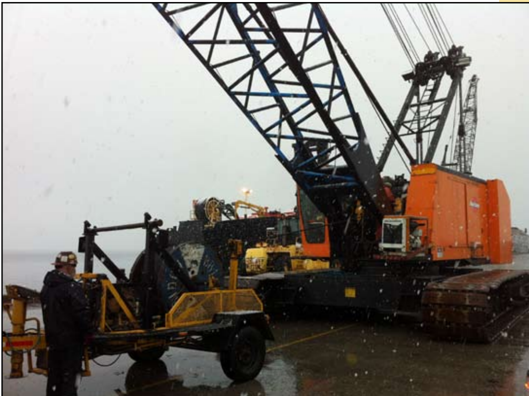
Changing the line on a North Star Stevedore crane at the Valdez terminal. John Bradshaw, John Mahan, and Mark Lindemann.
