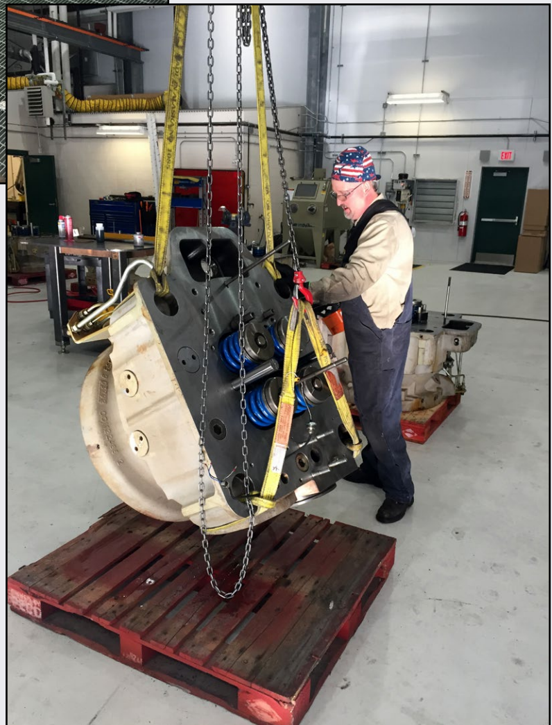
Maintenance Technician Ryan George working on one of the cylinder heads. Matanuska Electric Association (MEA)
