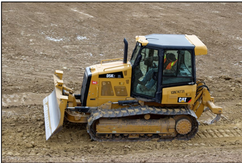
Apprentice Joel Oberdorfer learning to dress a slope in the dozer class.
