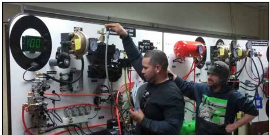
Mike Baker ( JCM Northlink) and Richard Kropp ( Deeny Construction) troubleshooting a brake problem on the Bendix EC-60 ABS/ACT/ESP Advanced Stability brake simulator at OE Regional Training at Bates Technical College.
