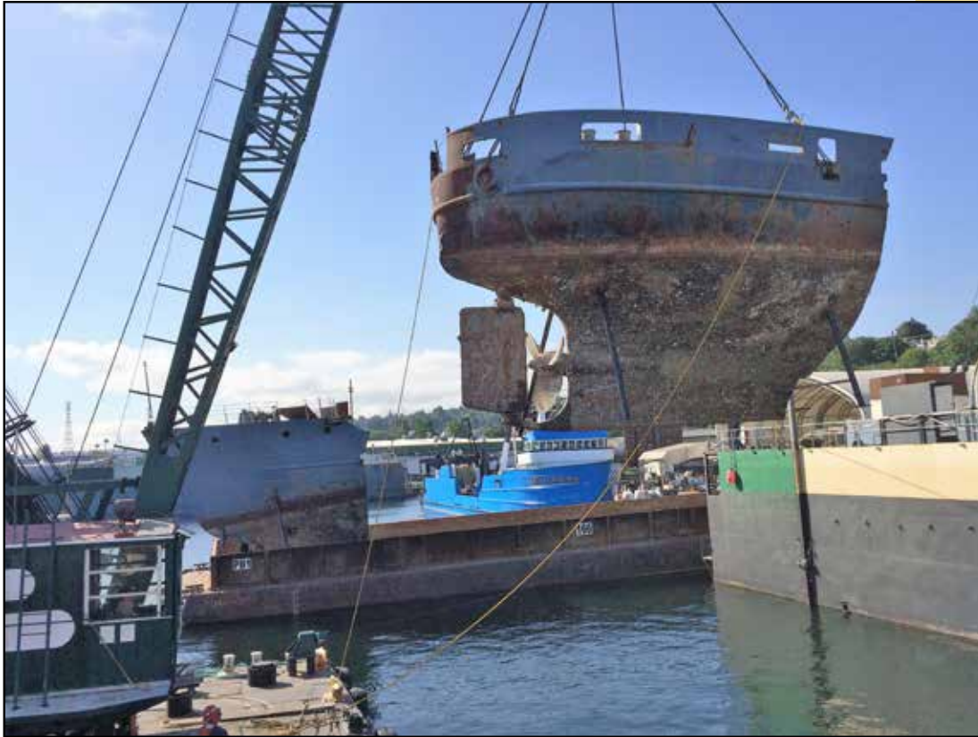
Mine Sweeper Stern at 63 tons
