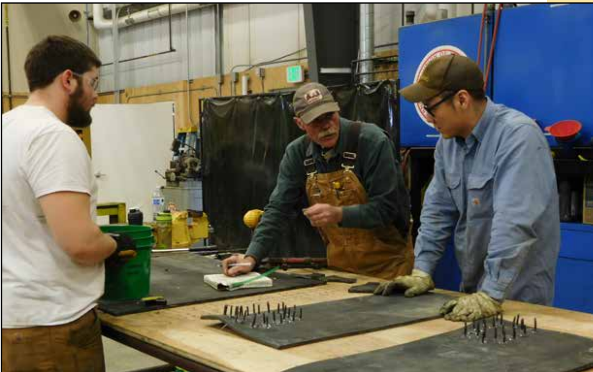
Instructor Al Odom gives advice to first year mechanics Josh Carson and George Mountain on patching and splicing conveyor belts.
