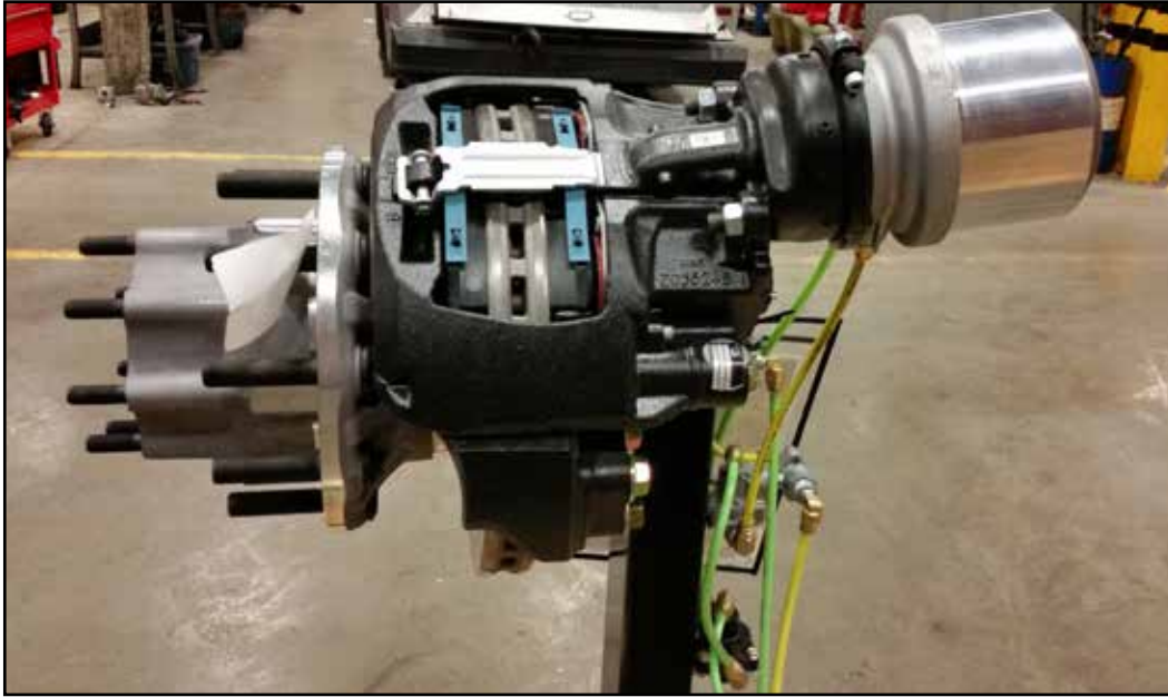
Bendix ADB22x Air Disc brake working mock up.
