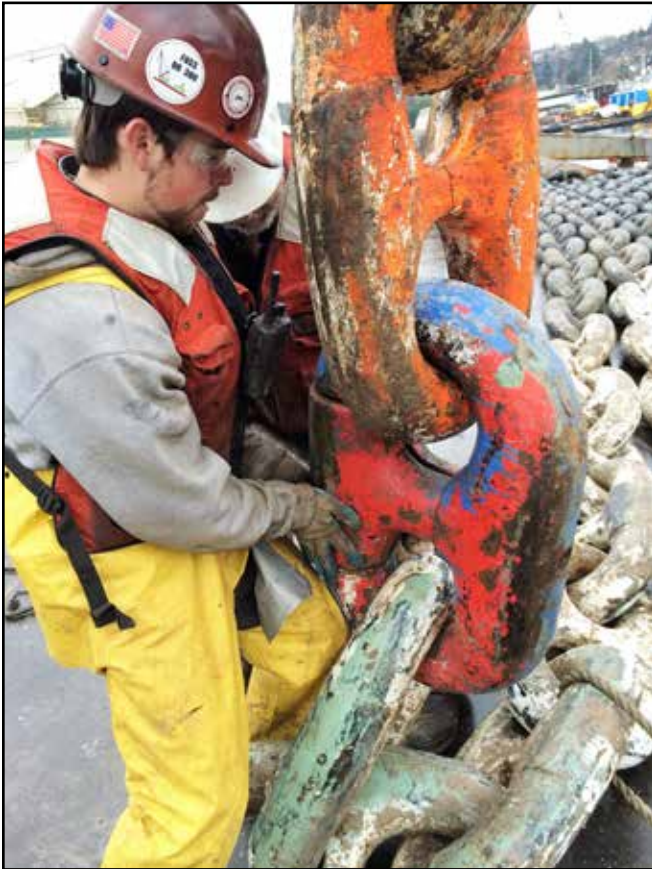
Jesse Tarabochia making up a connecting link for joining shots together.
